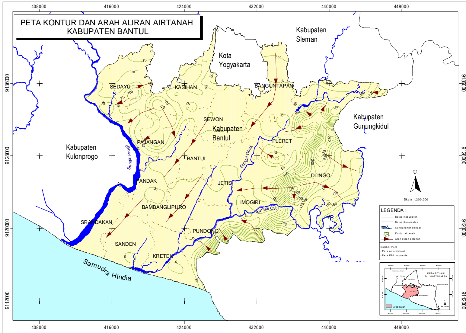
Lampiran (Appendix) 2. Peta kontur dan arah aliran air tanah Kabupaten Bantul (Groundwater contour and flow direction map of Bantul District)
