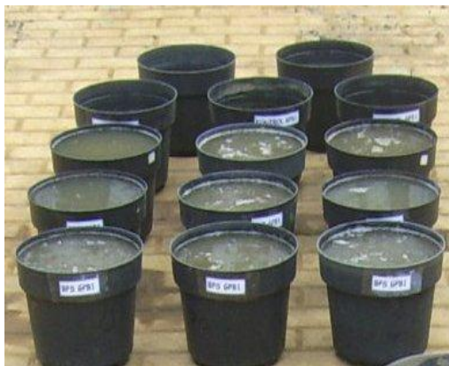
Gambar (Figure) 2. Ujicoba aplikasi inokulum BPS untuk menangani AAT di rumah kaca (kiri) dan di lapangan (kanan) ( Greenhouse trial of SRB inoculum (left) and field (right) to deal with acid mine drainage (AMD) )
