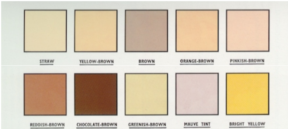
Figure 1. Color chart for the assessment and matching of colors in wood (Source: Ilic, 1990).
