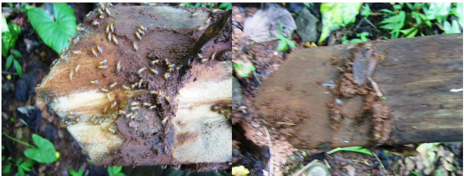
Figure 1. Test specimens after exposure to termites in the field trial for 6 months (Left: untreated test specimen infested by M. gilvus ; Right: treated test specimen remained sound).
