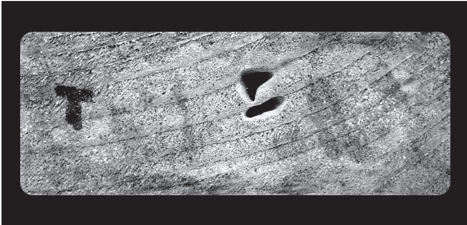
Figure 2. Slight damage to the exposed cut end of a bifenthrin-treated test specimen during the semi-laboratory trial with C. curvignathus .
